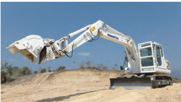
Machine developed based on hydraulic excavator (for processing unexploded ordnance)
