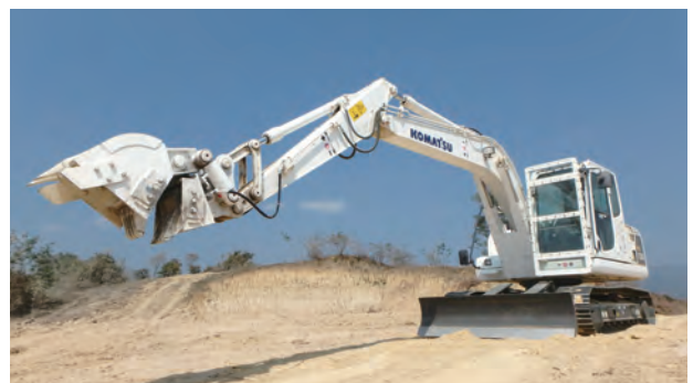
Machine developed based on hydraulic excavator (for processing unexploded ordnance)
