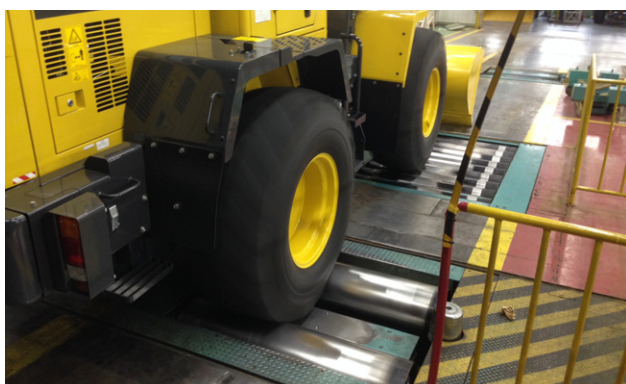
Brake test equipment
