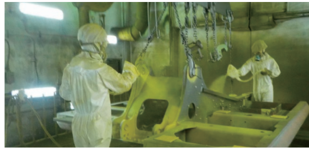
A painting operation at Osaka Plant using a paint having a high-coating efficiency
