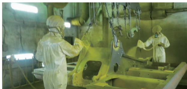
A painting operation at Osaka Plant using a paint having a higher coating efficiency
