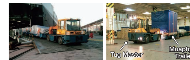
Press Units being loaded onboard; Loading onboard
