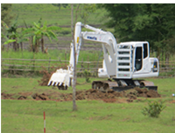
Demining machine (for handling unexploded submunitions) developed with hydraulic excavator PC130-8 as a base
