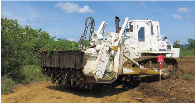
First model of the D85MS-15 demining machine being tested in Afghanistan
