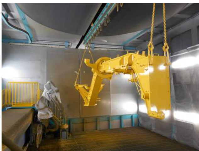
Frame coating with the coating robot
