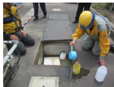
Water Quality Testing in Oily Water Separation Tank
