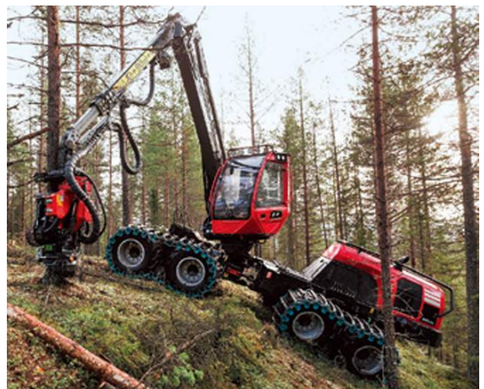
901XC eight-wheel ICT-equipped harvester
