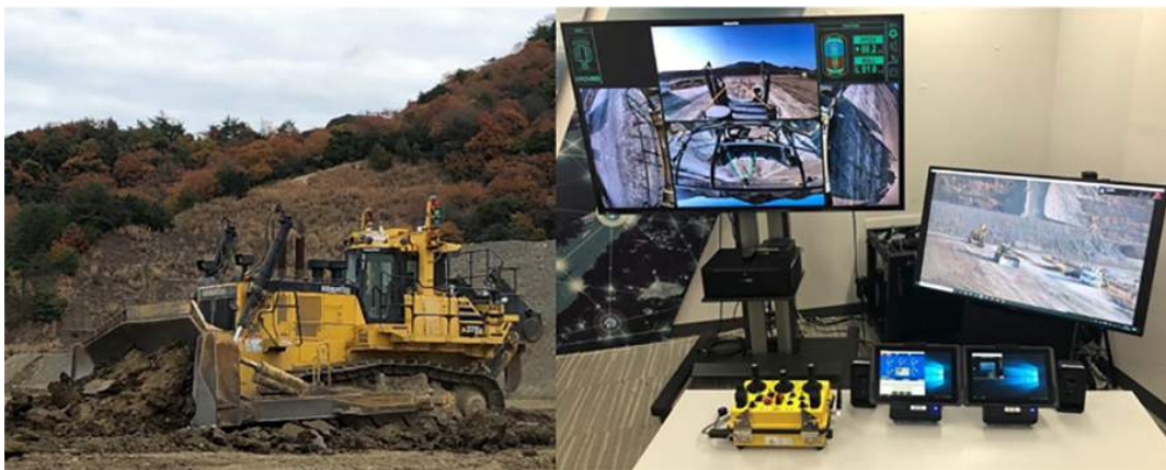
Remote operation of large-scale ICT bulldozer D375Ai-8 for mining using commercial 5G Left: Bulldozer located in Oita Prefecture Right: Remote control panel in Tokyo
