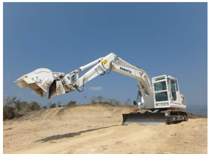
(2) Demining Machine for processing unexploded ordnance
