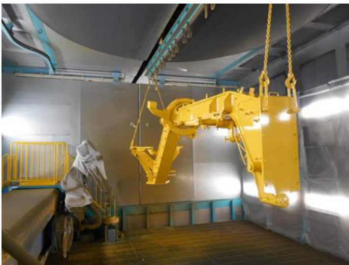
Frame coating with the coating robot
