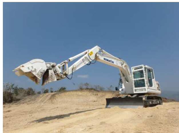
(2) Demining Machine for processing unexploded ordnance
