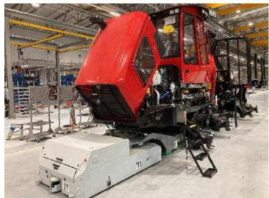
Forest machinery (Forwarder) on AGV
