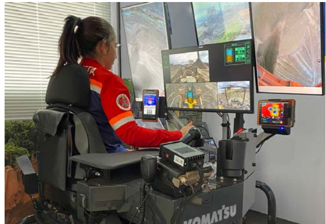
Remote control room that does not impair the operator's sense of control
