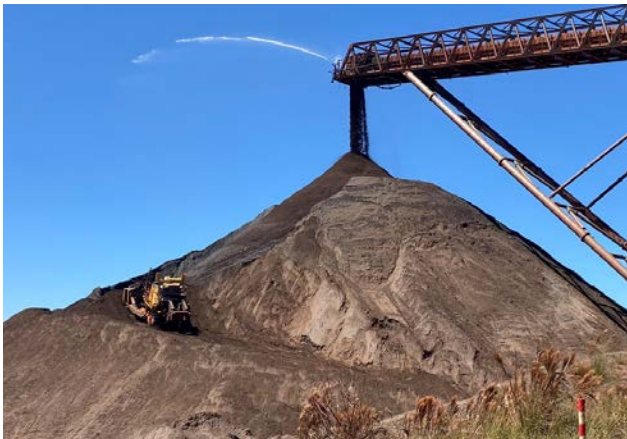
Remote-controlled bulldozer performing stockpile operations at the introduced mine
