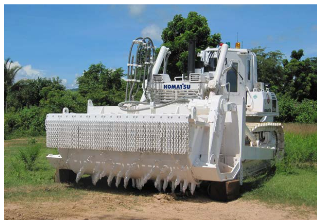
(1) Demining equipment for anti-personnel landmine
