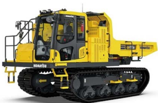
CD110R-3 equipped with a vehicle rollover warning system
