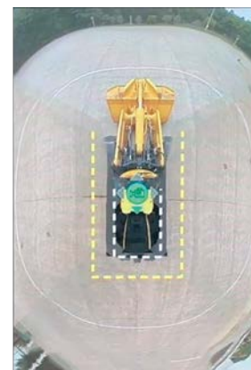
Bird's-eye view image of the WA470-11 wheel loader
