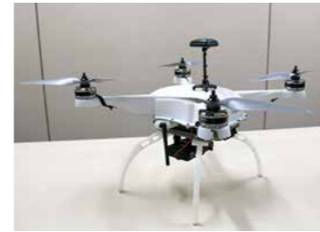
SMARTCONSTRUCTION uses Skycatch-made drone to survey the sites.
