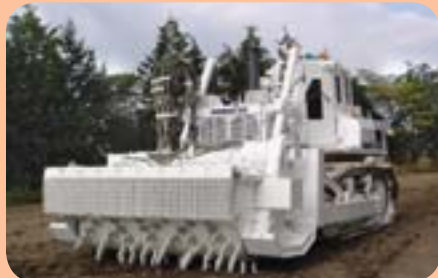
Komatsu’s D85MS demining machine for anti-personnel landmines
