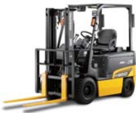
Hybrid electric forklift truck 2.5-ton model
