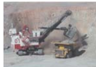
Autonomous dump truck being loaded with 300 tons of copper ore
