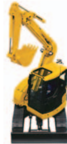
PC78UU hydraulic excavator with ultra-small turning radius
