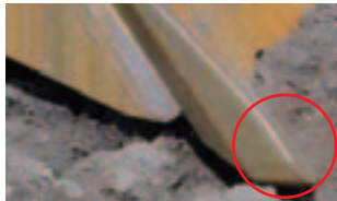
The thick tip encounters greater resistance in cutting
