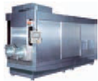
Wire saw for cutting solar cell wafers
