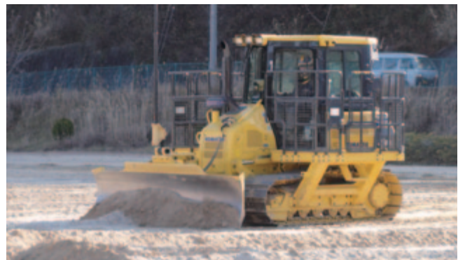
An Automated Machine Control/Guidance Bulldozer, Intended for Decontamination of Radioactive Material.
