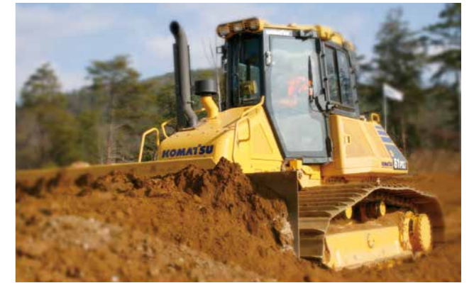
•• ICT-intensive Bulldozer D61PXI-23
